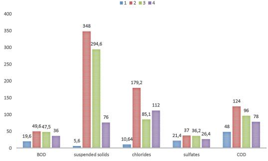
Figure 3. Dynamics of the content of pollutants in wastewater at the inlet and outlet of the existing treatment facilities of the bakery by BOD, COD, suspended solids, chlorides and sulfates; 1 – input (19.06.2020), 2 – output (22.07.2020), 3 – input (22.07.2020), 4 – output (04.12.2020)
