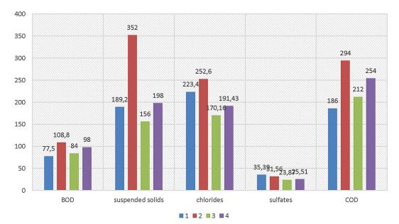
Figure 1. Dynamics of the content of pollutants in wastewater at the inlet and outlet of the existing treatment facilities of the cannery by BOD, COD, suspended solids, chlorides and sulfates; 1 - input, 2 - input, 3 - output, 4 - input
