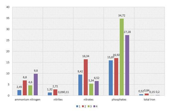
Figure 2. Dynamics of the content of pollutants in wastewater at the inlet and outlet of the existing treatment facilities of the cannery with ammonium nitrogen, nitrites, nitrates, phosphates and total iron; 1 - input, 2 - input, 3 - output, 4 - input
